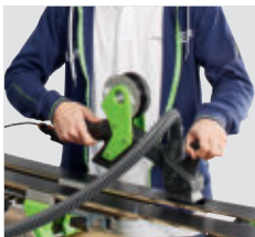
Melting head with larger contact surface, lower center of gravity and lighting for a better view of the melting area. Results: Tangibly improved control.
