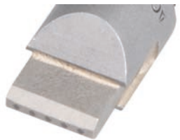
Diamond dresser Rhomboid 5 x 0,6 x 0,6 mm, Total bearing surface 1,80 mm², r = 0,40 mm
