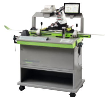
Safetronic Ski Binding Testing and Adjustment Machine
