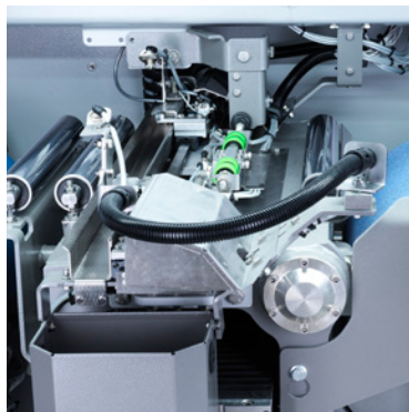
Trim Cut for automated sidewall removal
